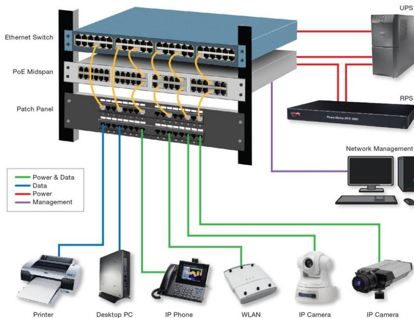
Fig. 2: Midspans decouple the power and data infrastructures.
