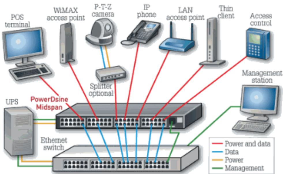
Fig. 1: PoE midspans are installed between the network switch and PDs.
